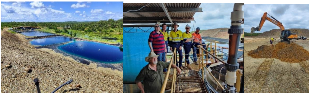
Figure 3 – 3(a) PLS ponds containing residual copper, 3(b) Metallurgical and electrical team on site with R3D personnel, and 3(c) Sampling the heap leach material to upgrade the resource status and conduct further metallurgical test work.
