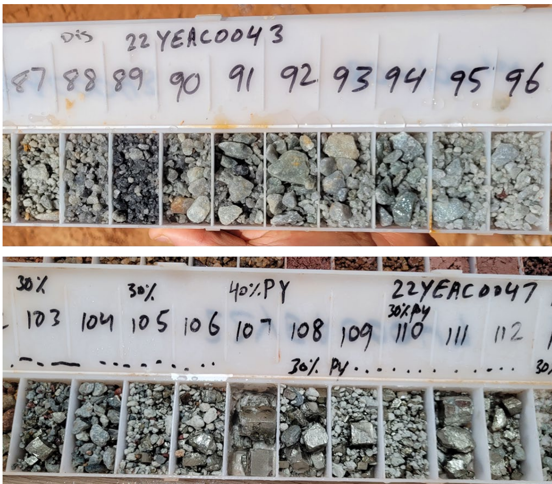
Figure 3: Air core chips from Mistletoe showing intense alteration and pyrite
