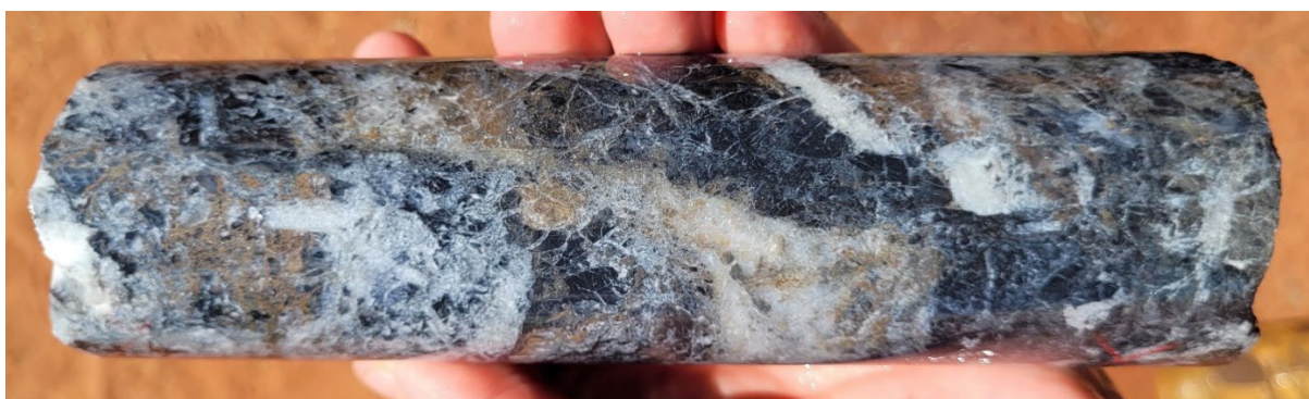
Figure 1: Intergrown barite-sphalerite-galena associated with brecciated and chlorite-carbonate-silica altered mafic volcanics and shales (21YERD0016, 372m)
