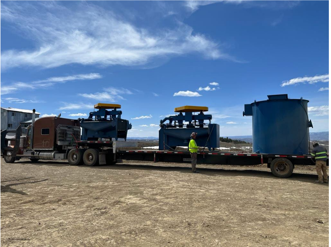
Figure 1 250tpd flotation cells and conditioning tank delivered to site on April 19
