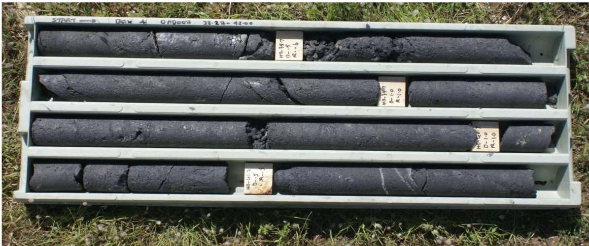
Figure 2: High-grade graphite drill core from the Oakdale Graphite Project – 36.2m to 42.2m @ 19.71% TGC 7
