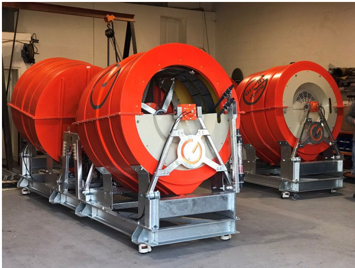
Multi Gravity Separators at the factory awaiting shipment and installation at the Dolphin Tungsten Mine
