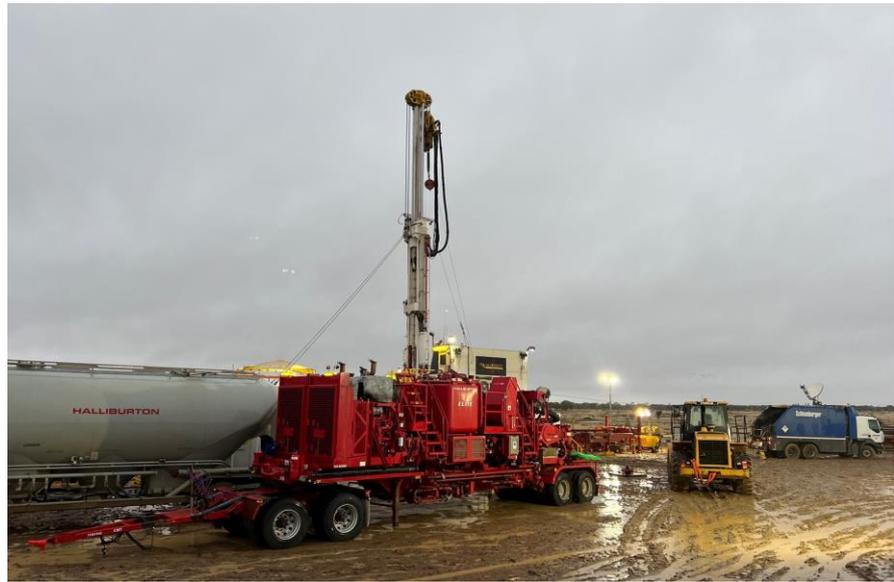
**Figure 2:** Wireline and cementing equipment at Glenaras 24
