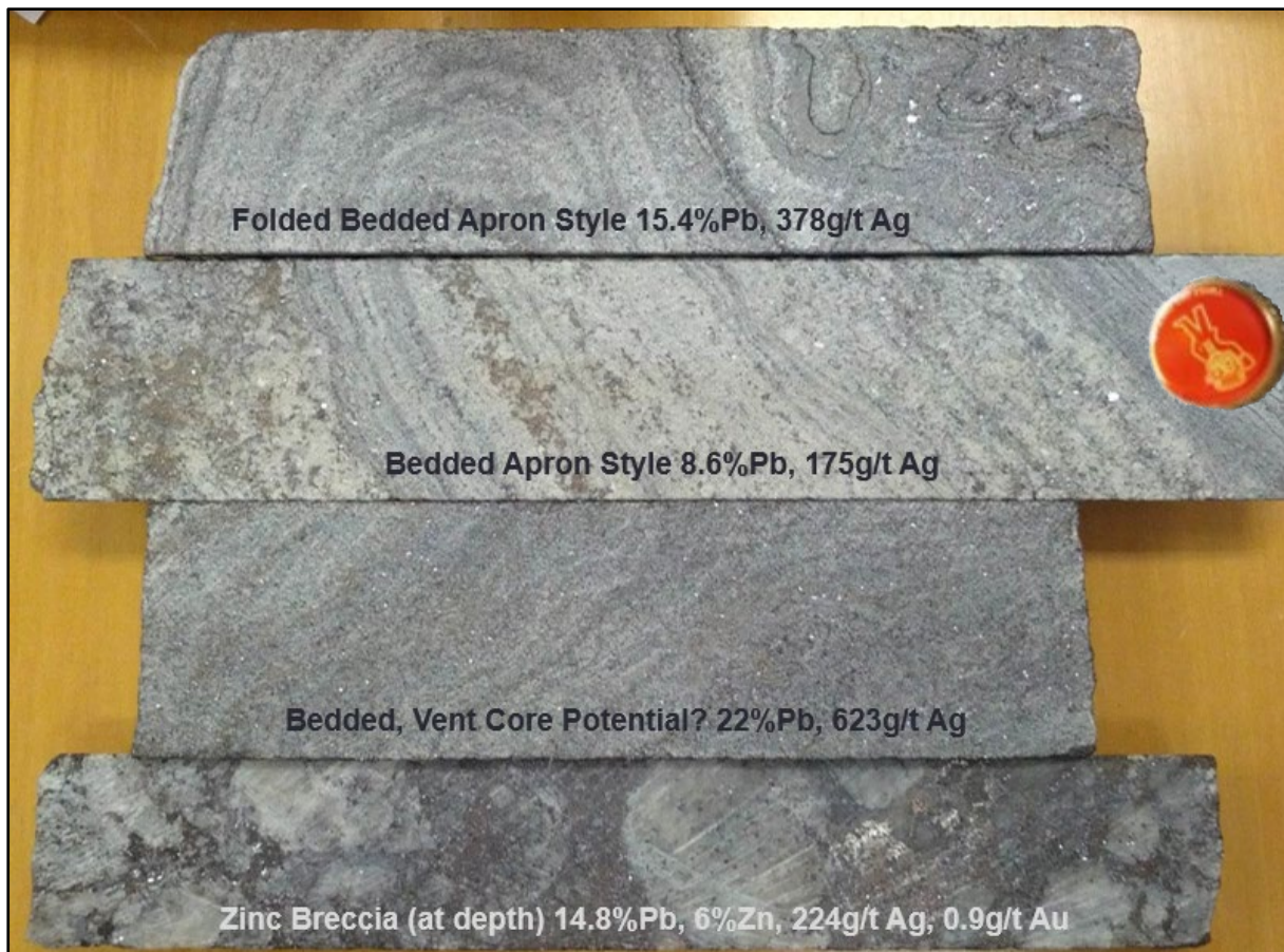
Figure 14: Examples of sulphide textures and grades
