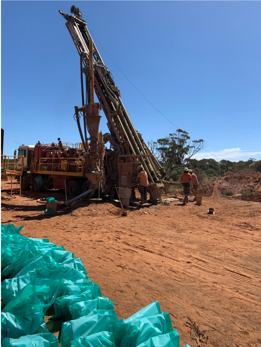
Figure 8: Photo of RC drill rig at Apollo with drill chip samples being collected.
