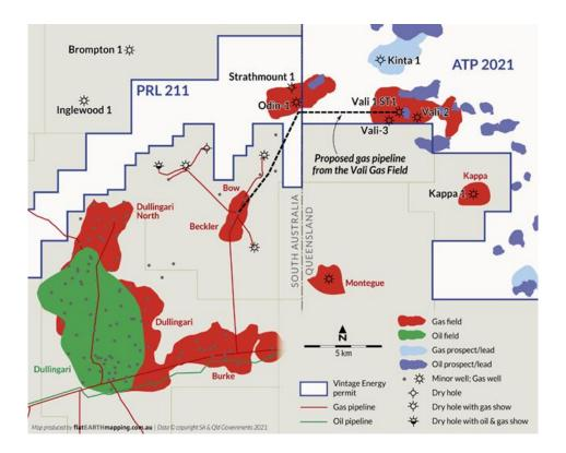
The field has three cased wells which are to be completed and connected to the Moomba gas gathering network for supply to the eastern Australia domestic energy market. Vali-2 and Vali-3 are to undergo fracture stimulation of the Patchawarra Formation prior to completion.
