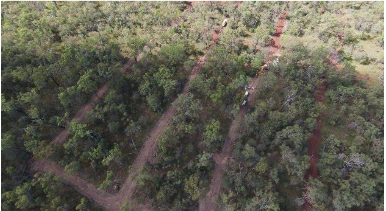
Figure 4 drilling grid tracks at Gunnawarra
