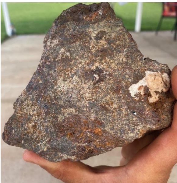
Figure 4: Photo of sample MNRK0529 (39.7% TREO, 6.30% Nd 2 O 3 +Pr 6 O 11 ) showing large reddish brown monazite crystal masses within an ironstone vein from near Y3.
