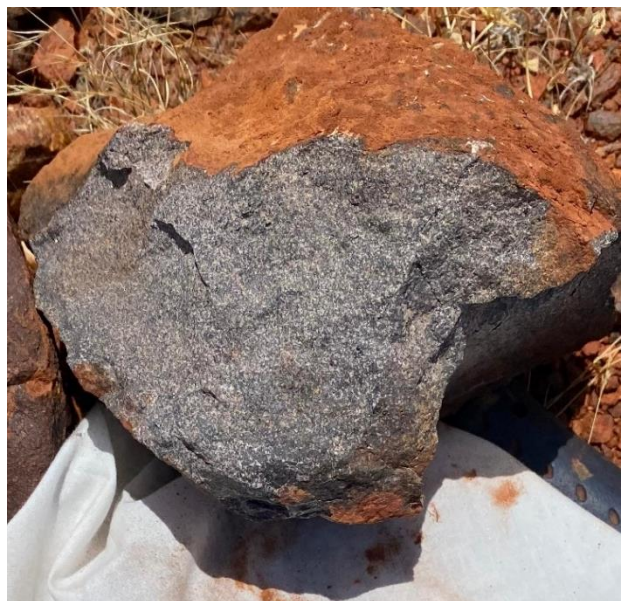
Figure 5: Photo of a niobium vein (MNRK0527 (5.8% Nb 2 O 5 , 0.35% TREO) from near Y3 comprised of quartz, ferrocolumbite, hematite and magnetite.
