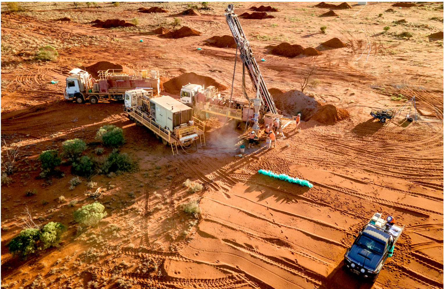
Figure 2: RC Drilling underway at Aurora Tank (April 2022)
