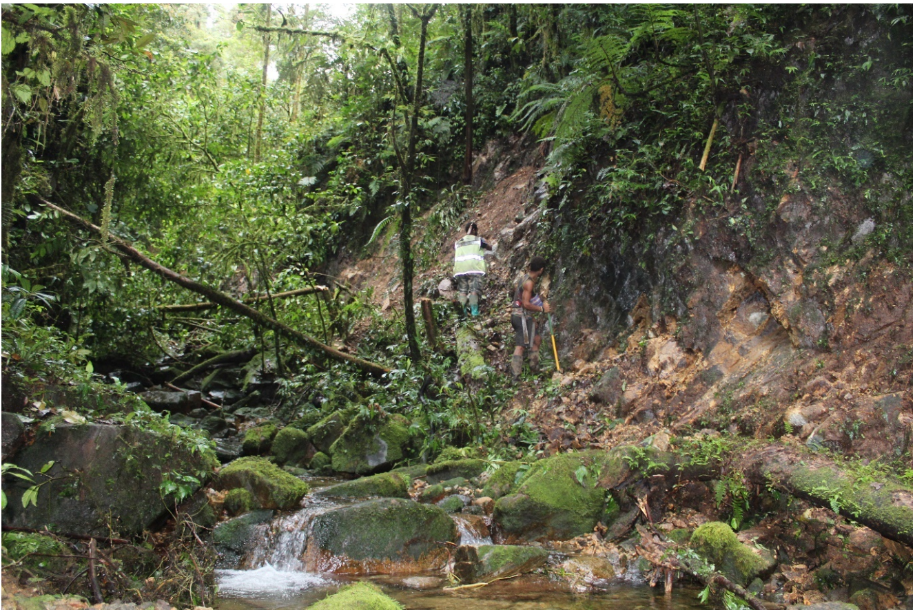
Figure 4. Zones of endo-skarn with minor (1%) malachite staining, a grab sampled # MWR 166 assayed 1.4% Cu and 2g/t gold.
