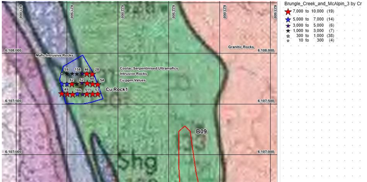
Figure 17: Cu Rock 1 Prospect chromium in coloured stars and copper as numbered analyses
