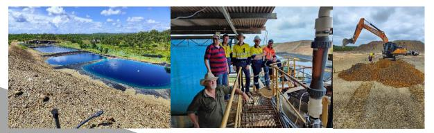
Figure 3 - 3(a) PLS ponds containing residual copper, 3(b) metallurgical and electrical team on site with R3D personnel, 3(c) Sampling the heap leach material to upgrade the resource status and conduct further metallurgical test work.
