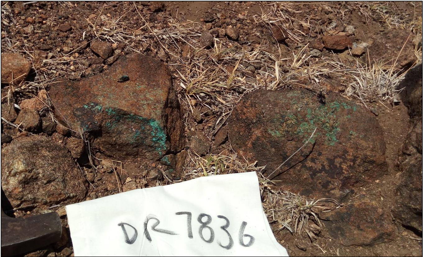
Fig. 20 Main Top diggings - discarded low-grade material assayed 0.43% copper and 0.35 g/t combined gold platinum palladium. CML is targeting a very large tonnage of similar grade, with included higher grade layers.
