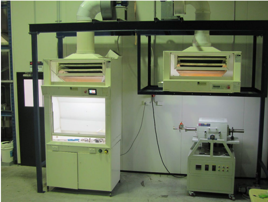
Customised reactor for recovery of fluorine from aluminium smelter bath
