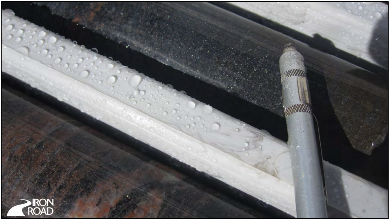
NQ2 diamond core stored in core tray- very coarse-grained magnetite gneiss.
