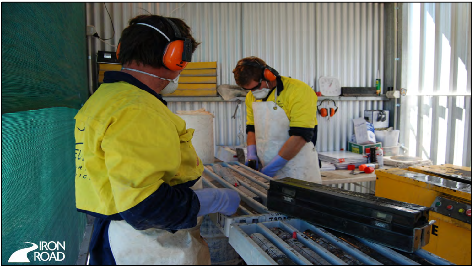
NQ2 diamond drill core was split using an automated diamond core saw with one half retained and the other half sent to the mineralogical laboratories for assay using XRF techniques for an iron ore suite of 26 elements.
