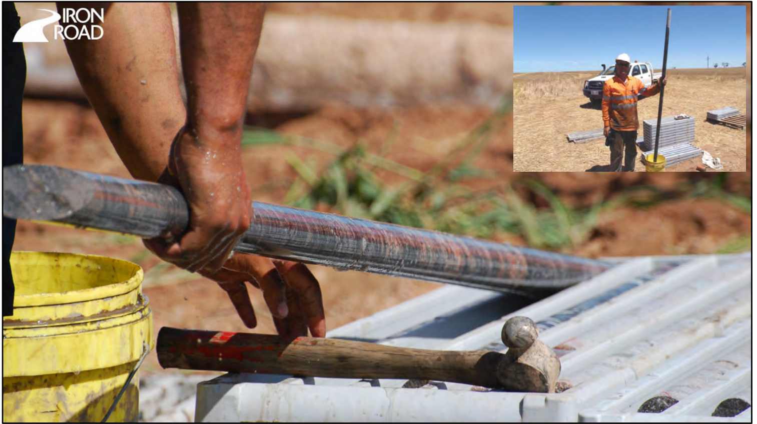
Diamond drill core being placed in core tray by driller. Rock Mass Quality (RQD) is excellent with recovery of long continuous core runs common.
