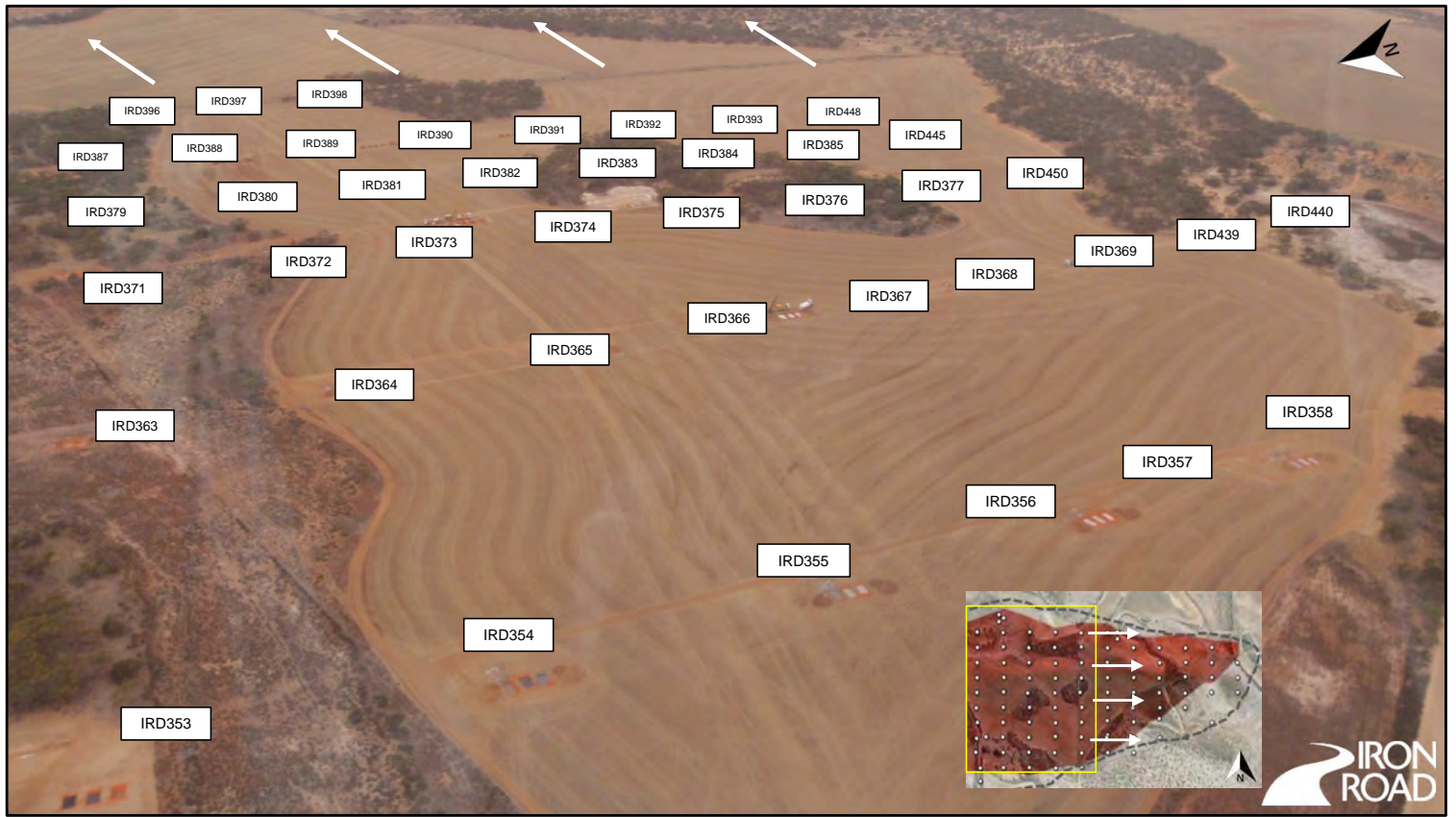
Representation of drill collar ID's with drill lines advancing from west to east (December 2011).
