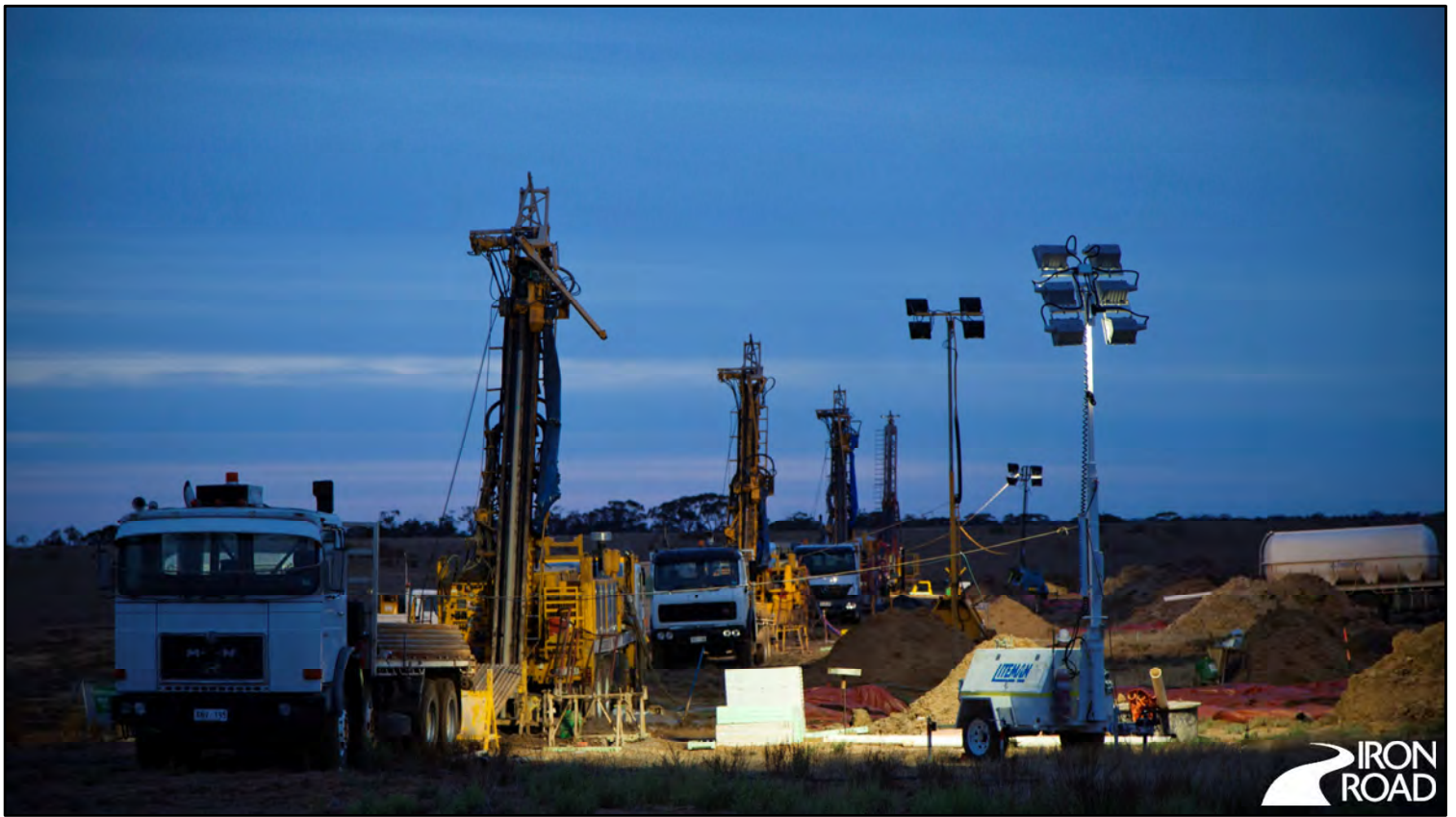
Tighter drilling pattern of 100x50m utilising four diamond drill rigs to allow for a representative variography model to be constructed for Mineral Resource estimation.
