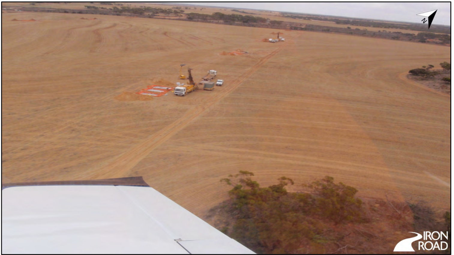
Diamond drills on north-south traverse. Almost all drilling was oriented at -60^\circ true north (December 2011).
