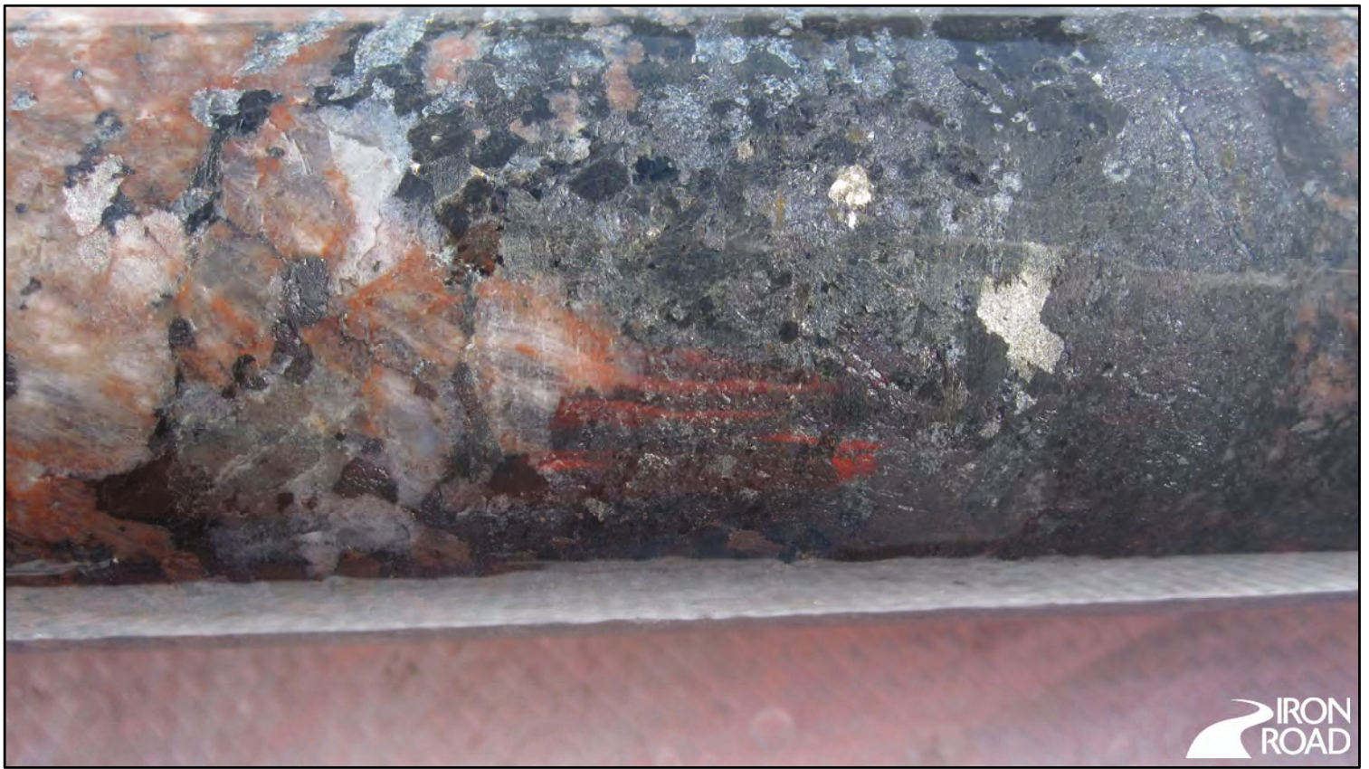
Very coarse-grained magnetite gneiss. Note the granular texture of gneiss.
