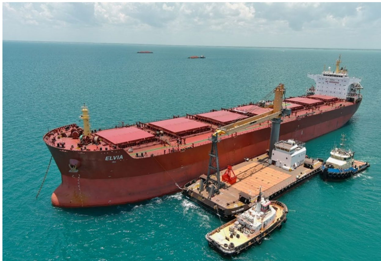
Figure 1 Prepositioning of floating crane to commence loading activities
