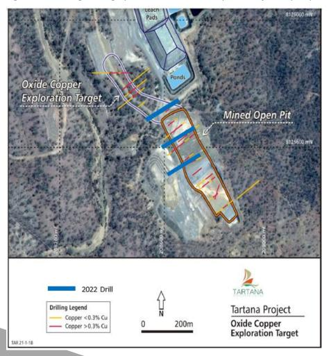
Figure 3 – Location of three drill lines and surrounding infrastructure including heap leach pads and partially rehabilitated open pit. Drill section lines represented by the blue lines.
