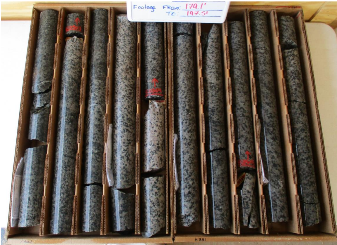
HC22-OM02: clinopyroxene quartz monzonite w/ lesser clinopyroxene quartz monzosyenite from 179.1-197.5 ft depth
