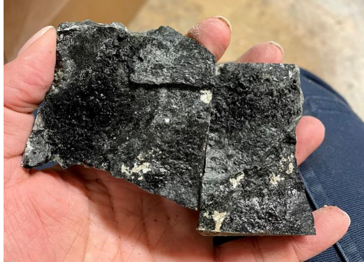
HC22-RM02: Image of possible allanite vein analyzed by handheld XRF
