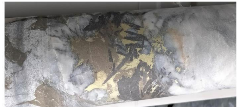
Intergrowth of wolframite and chalcopyrite in broad mineralized zone (EQ026, 93.2ms)
