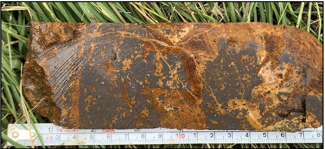
Photo 3: Mayfield brecciated magnetite skarn in drill core MA13, 99m
