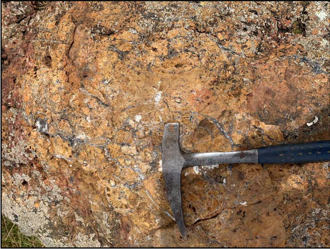
Photo 4: Mayfield prospect brecciated skarn with chalcedonic veins
