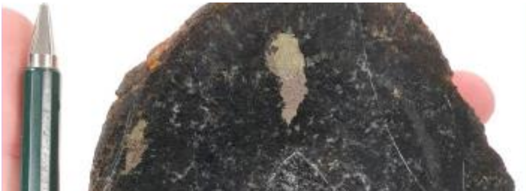
Figure 3: A cut slab through rock chip GLRK008 showing multiple blebby three-phase magmatic sulphides within the Money Intrusion.
