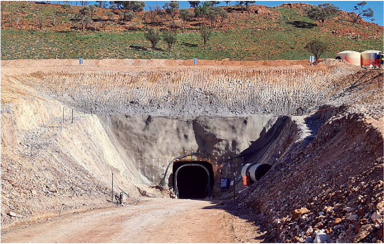
Figure 2 – Pyrite Hill decline heading as shown currently developing through unmineralised waste material in the hanging wall of the deposit with mineralisation expected to be intersected during May.
