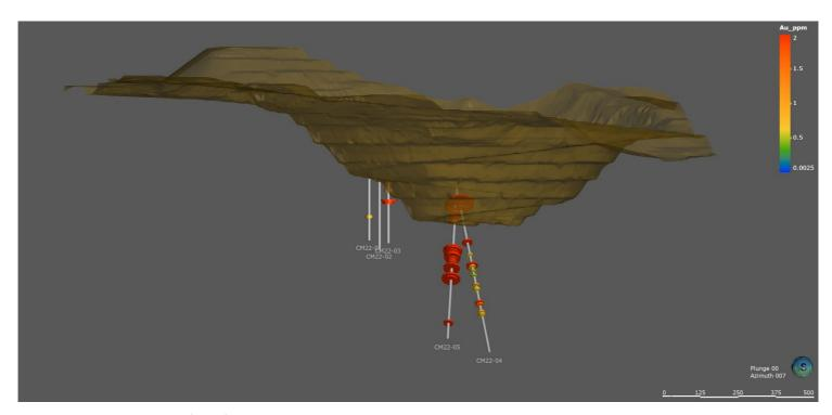
Figure 1: Cross Section of the five completed drill holes with assay results. View looking north, Azimuth 005
