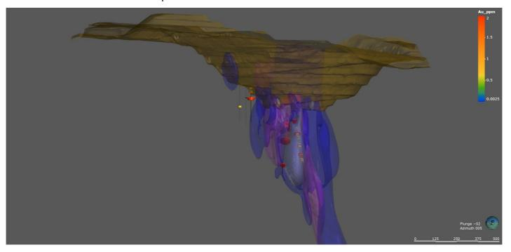
Figure 2: Cross Section of the five completed drill holes with potential for deeper extension of the mineralised ore zone
