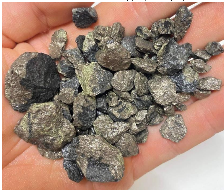
Figure 1: RC chips from REYRC002 80-81m showing net-textured / brecciated Ni-Cu sulphides (~15-20%) comprised of pyrrhotite, chalcopyrite and pentlandite.
