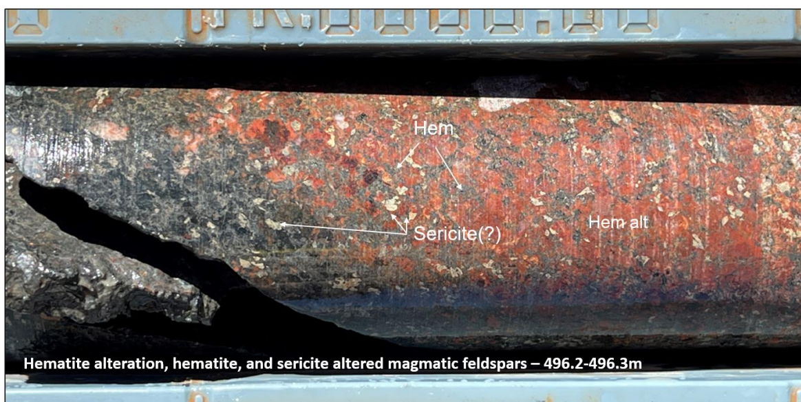
Figure 9. Photo of hematite altered host intrusive. Hematite occurs as red staining of the host rock and as hematite disseminated throughout the matrix. Igneous feldspars (plagioclase) are altered to sericite(?). Photo is of NQ ½ core (Ø = 47.6 mm).
