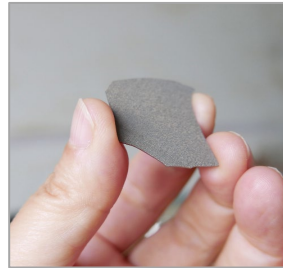
High-purity electrolytic manganese metal (HPEMM >99.9% purity)
