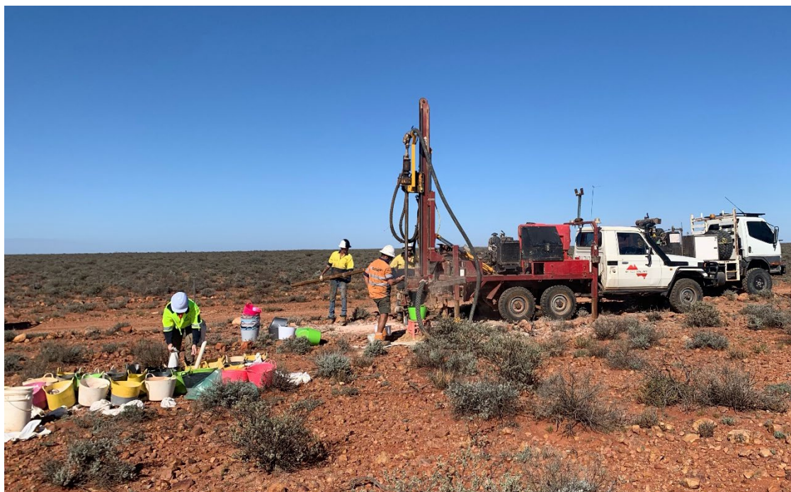
Photo Air Core Drilling Operations Underway at Comet
