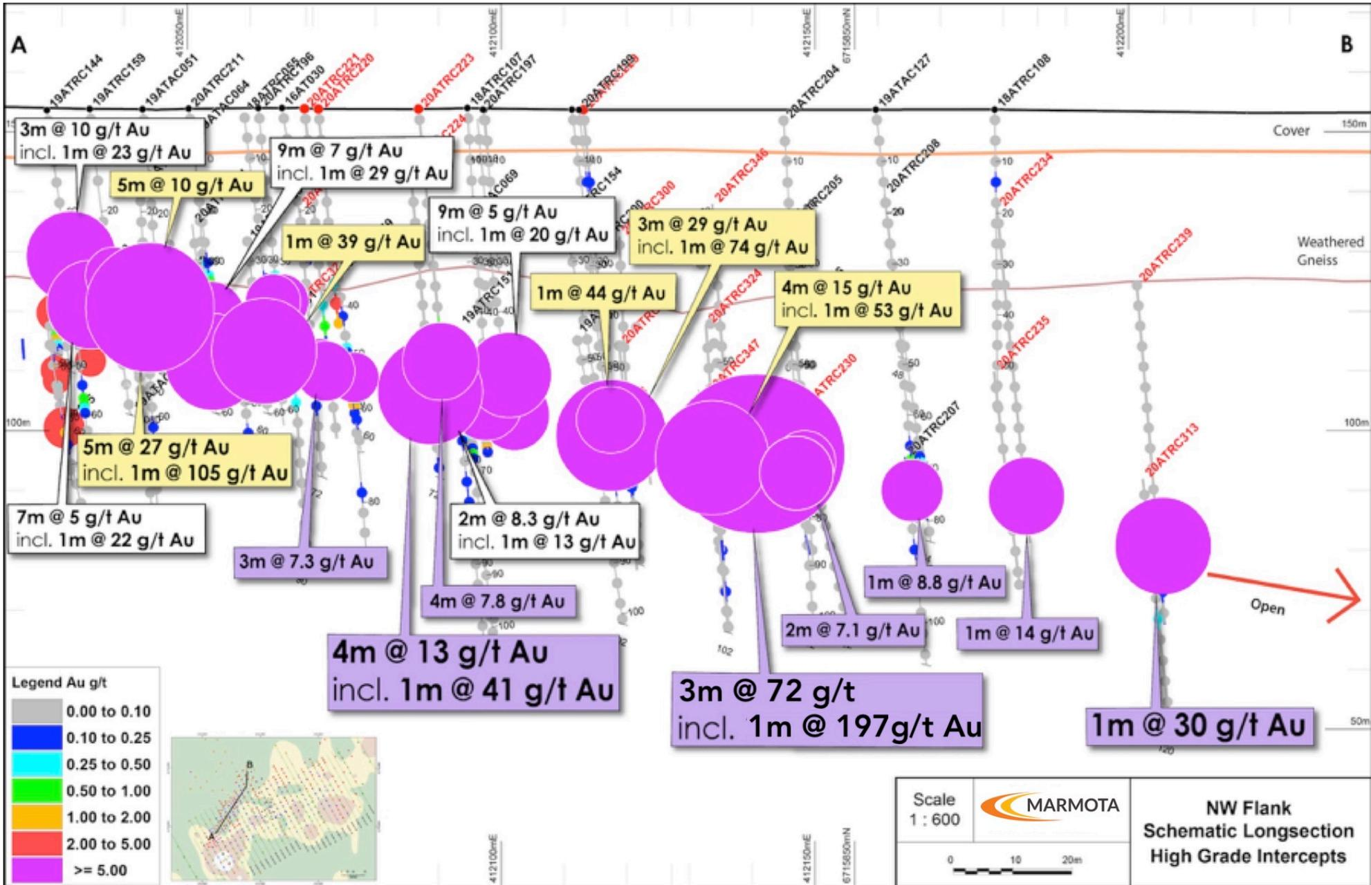
Figure 3: Schematic long-section through new NW flank
