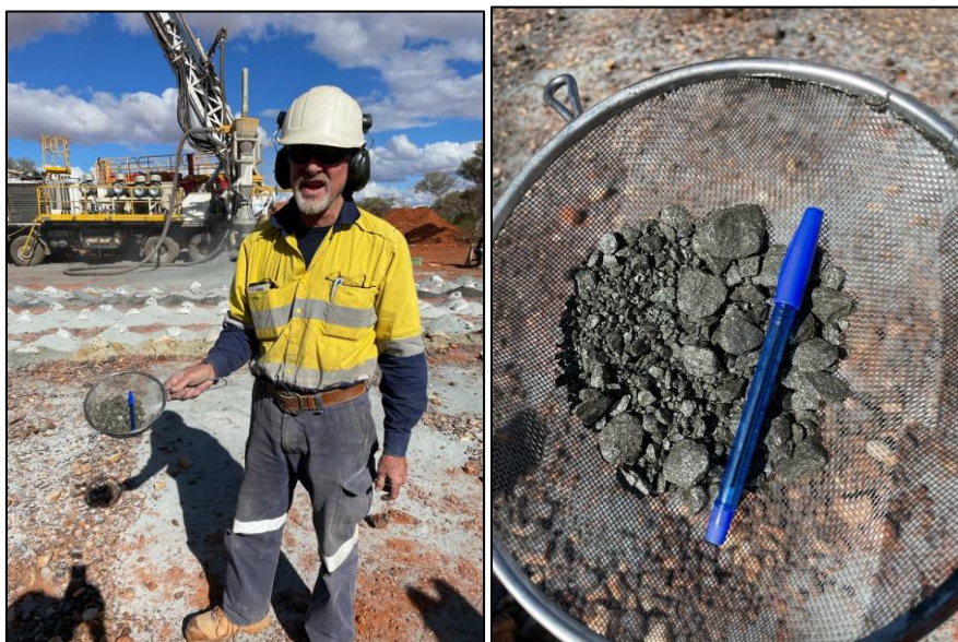
Figure 2 – RC Drilling and sieve with semi-massive pyrite mineralisation
