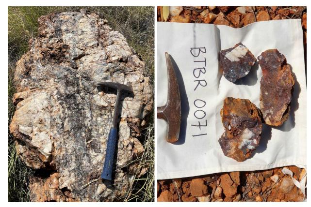
Plate 3: Eastern vein outcrop showing multiple episodes of fracture and veining (LHS); sample BTBR0071 from this location returned 17.1g/t Au (RHS).
