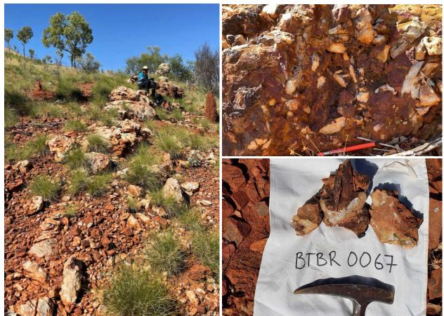
Plate 1: Western vein outcrop (LHS), complex brecciated quartz (top right); sample BTBR0067 returned 6.04g/t Au (bottom right).
