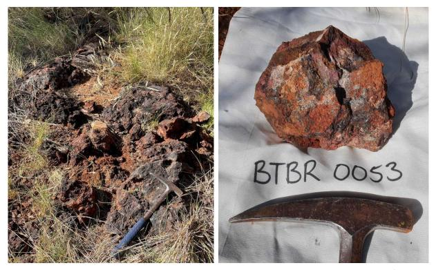
Plate 2: Gossan – south of Duck Creek Fault (LHS); sample BTBR0053 from that location returned 10.25g/t Au (RHS).
