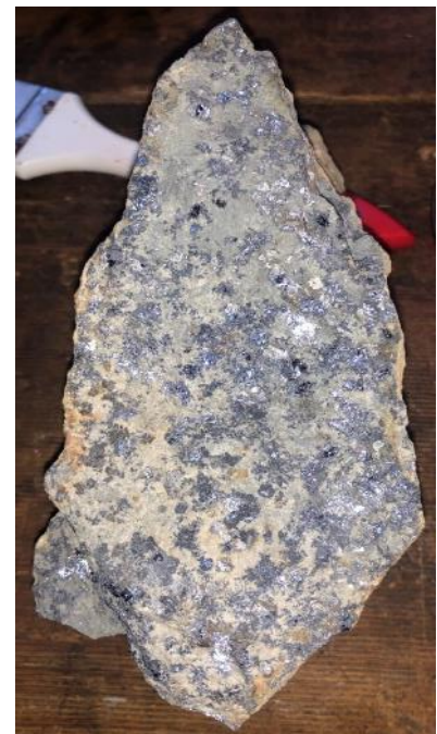
Photo 4: Webbs Consol Main Shaft specimen showing coarse galena mineralisation
