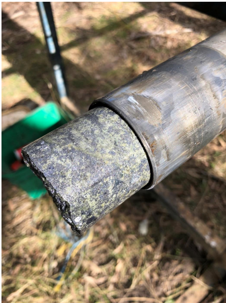
Photo 3: Very coarse blebs of galena (PbS) in WCS019 drill hole core barrel (NQ2 core size)
