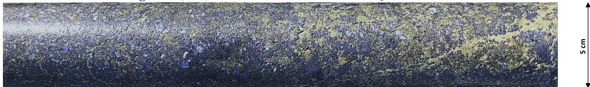
Photo 1: Coarse blebs of galena (PbS) in core from drill hole WCS019
