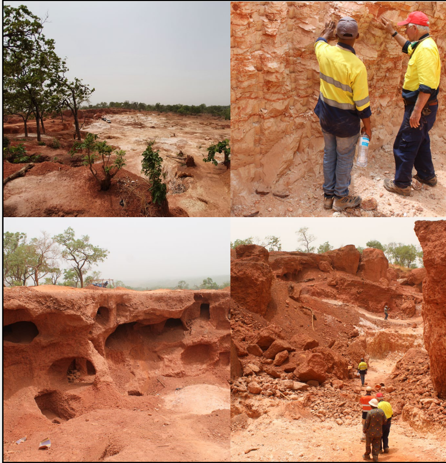
Alahiné artisanal gold workings typically range 5-15m in depth targeting mineralised laterite, near surface supergene gold. Main mineralised trend hosts >4km of artisanal workings.
