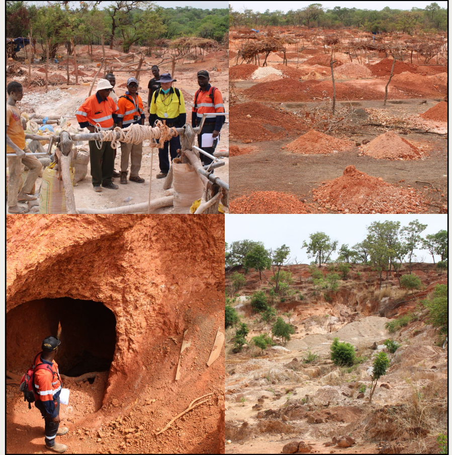
Mansala artisanal gold workings in "Area F" within NE quadrant of licence typically comprise shallow pits and prospecting shafts across estimated >600m strike.
