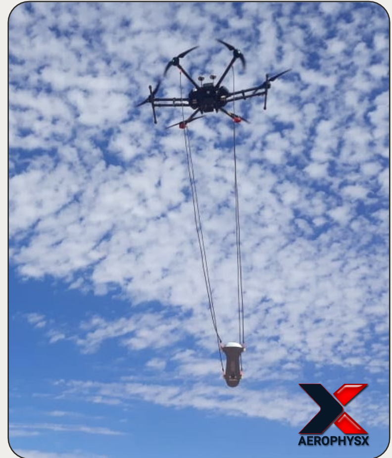
The AeroPhysX UAV airborne magnetic survey system in operation at the Alahiné Gold Project.
