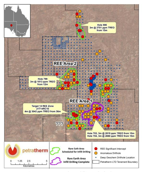
Figure 1 Comet REE Project showing drilling completed to date.
