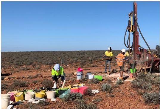
**Photo** Air Core Drilling Operations at Comet
