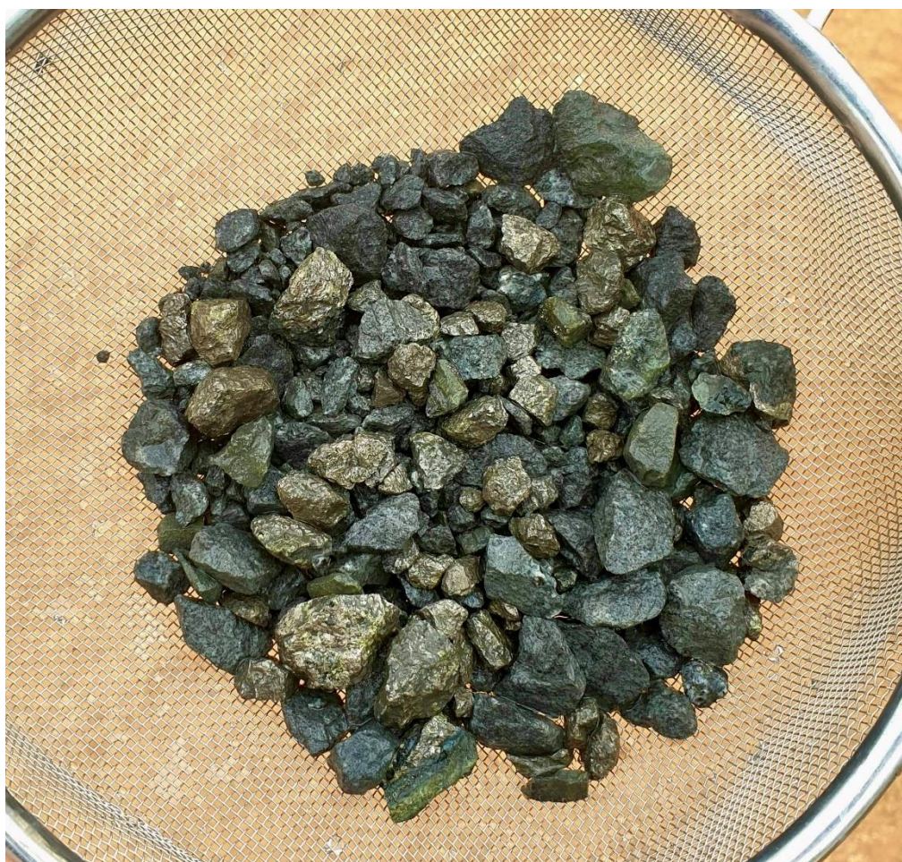
Figure 3: RC chips from REYRC002 79-80m showing net-textured / brecciated Ni-Cu sulphides (~15-20%) comprised of pyrrhotite, chalcopyrite and pentlandite.
