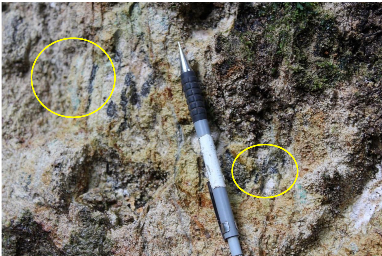
Figure 4. MWTR008, clay-limonite – haematite – manganese alteration containing chalcocite and malachite (Circled)
