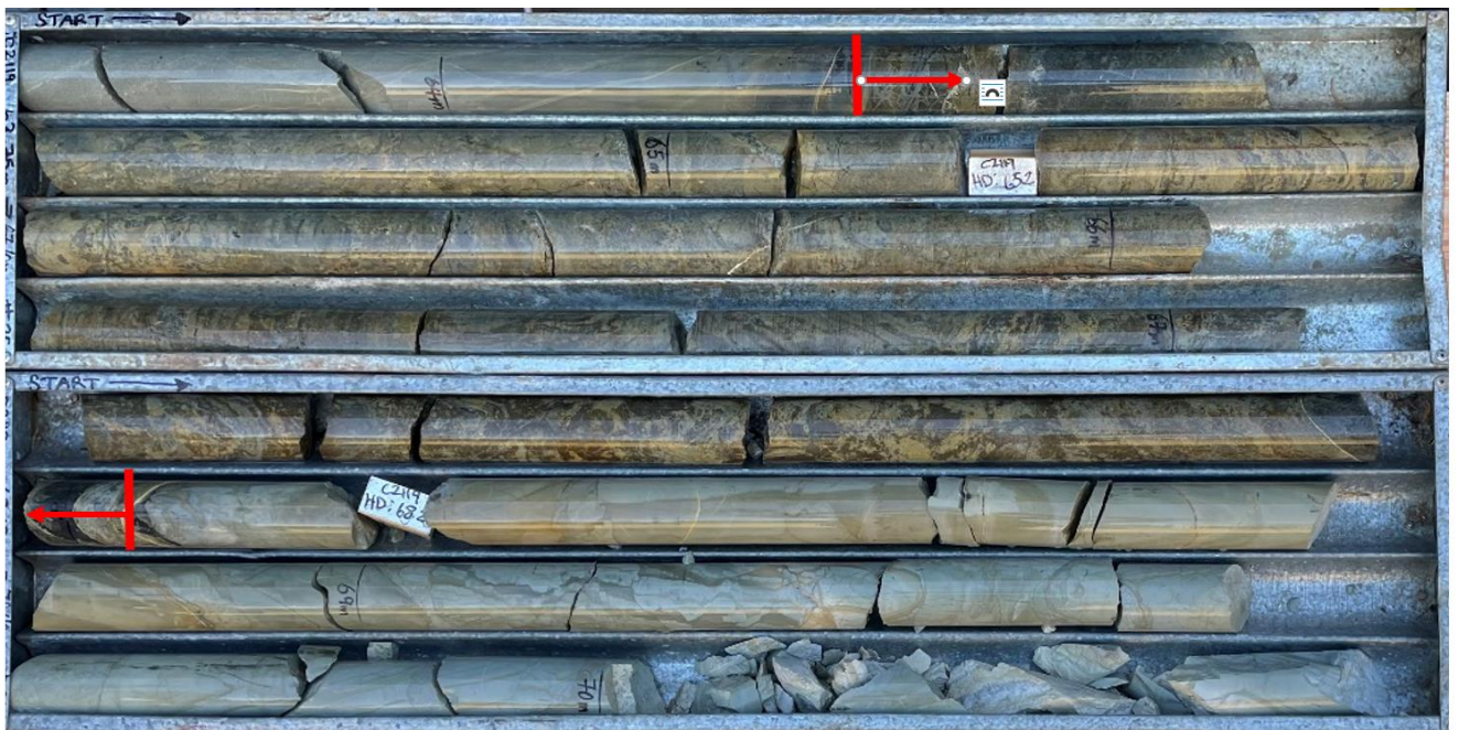
Figure 5. C2119 – NQ core from Battery Lode mineralisation intersected from 64.3m for 3.7m (red arrows identify sample interval).
