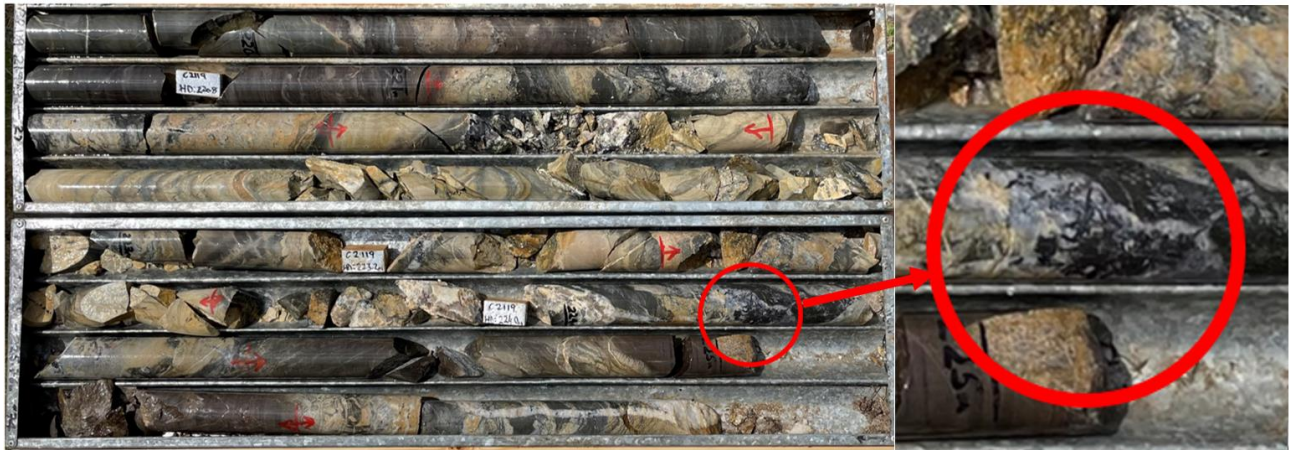
Figure 7. C2119 – NQ core depicting Intensive quartz fissure vein and silica/muscovite/sericite alteration from the Foley's Zone. Visible coarse wolframite (circled), plus fluorite and molybdenite at 224.3m. (red arrows identify sample intervals).
