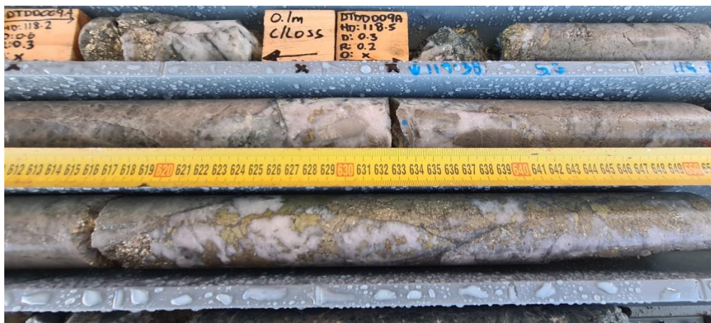
Figure 4 - DTDD009 118 - 121m Showing Significant Quartz-Chalcopyrite Veins
