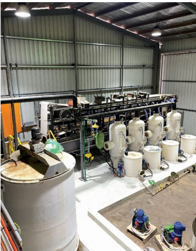
Figure 5 – Broken Hill plant. Left: Horizontal vacuum filter belt. Right: Pressure oxidation leach circuit.
