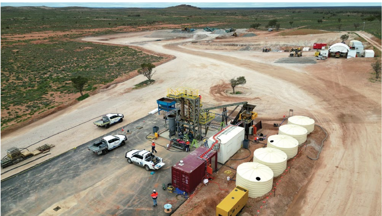
Figure 3 – Pyrite Hill site concentrator including gravity spirals.
