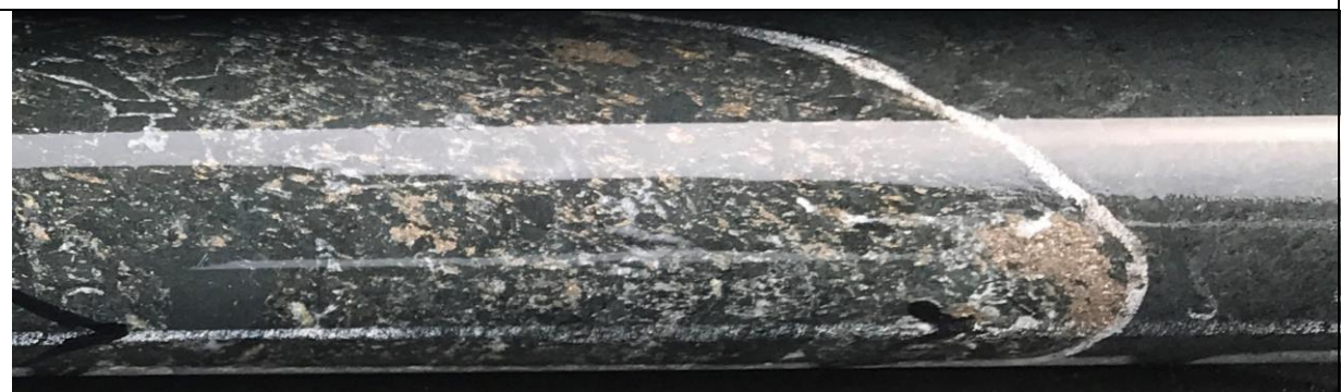
Figure 11: LBSDD002 – 208m - Mafic breccia in contact with a fine to medium grained clinopyroxenite with strongly disseminated to matrix magmatic sulphide on the contact. Field of view from top to bottom ~ 36mm.
