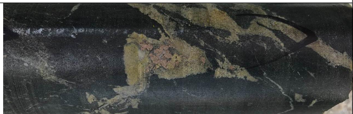
Figure 10: LBSDD001 – 94m – fine-grained melanogabbro with an irregular syn-genetic feldspar tremolite vein with blebby magmatic sulphide. Field of view from top to bottom ~ 47mm.
