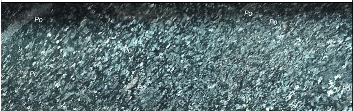
Figure 4: LBNDD001 – 246.00m – blebby magmatic sulphide mineralisation associated with a feldspar vein in a medium to coarse grained granular clinopyroxenite. Field of view from top to bottom ~30mm.
