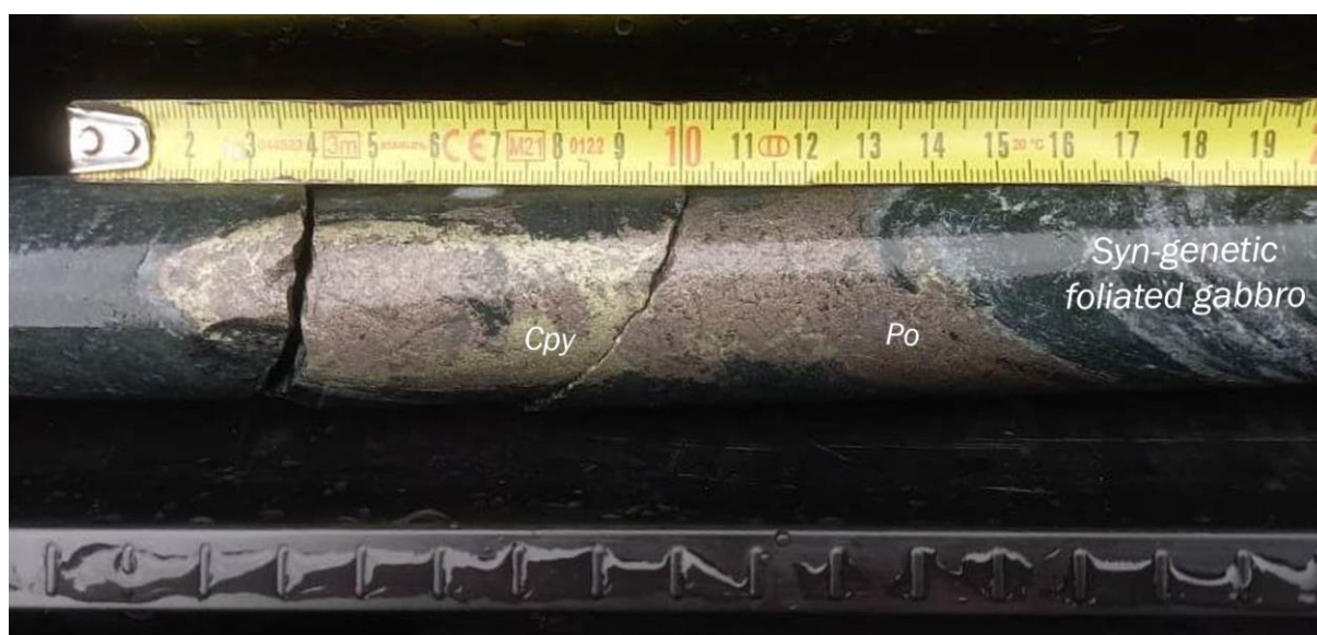
Figure 1: LBSDD001 – 141.96m – 142.07m – magmatic sulphide stringer mineralisation, chalcopyrite (Cpy) and pyrrhotite (Po), within a gabbroic unit.
