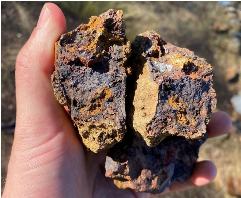
Figure 1: Recently discovered gossanous rock chips with boxwork textures after sulphides from the ~700m x ~100m OR4 anomaly associated with a ~500m x ~370m x 3,300S FLEM conductor.
