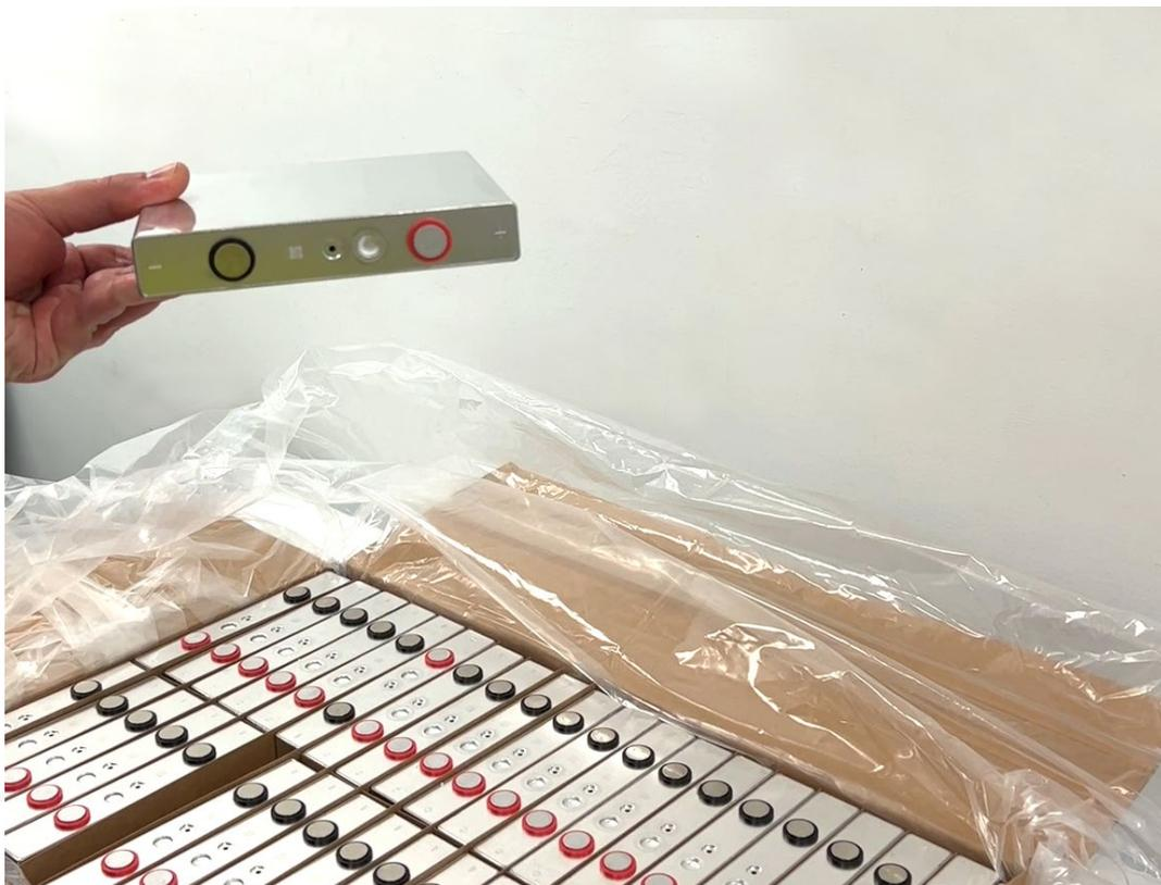
**Figure 4: Battery cells produced from semi-automated production**
