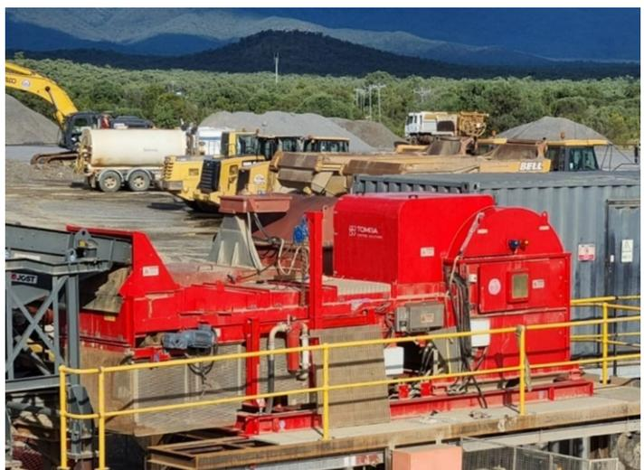
Fig.1 – 2<sup>nd</sup> TOMRA XRT Sorter (both XRT Sorters can operate in parallel or individually, utilising same product and waste conveyors)
