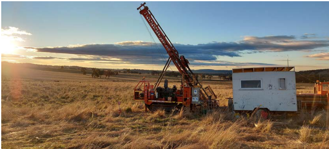
Figure 1. Diamond drill rig at the Barabolar Project.
