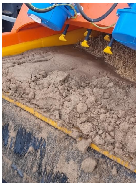
Figure 3. Ardmore Phosphate Rock Mine - Final Screen (Wet Product), Beneficiation Plant
