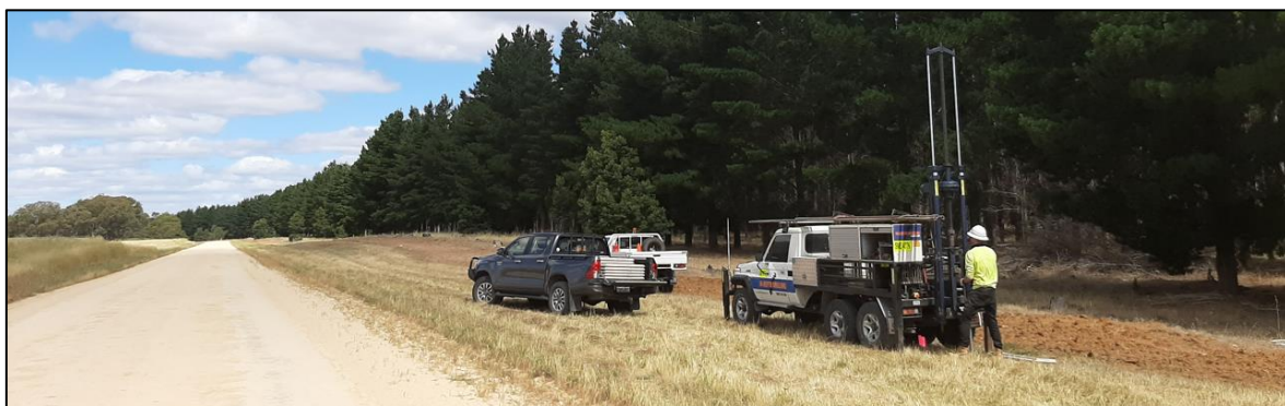
Figure 3 – Push Tube/core drilling in progress
