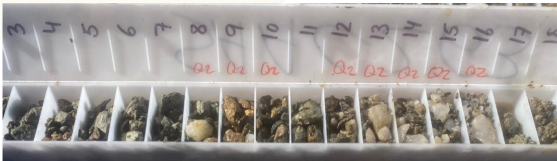
Figure 3: Photograph of aircore chips showing extensive quartz veining at the Overdrive prospect in SAAC0263 from 2-18m. NB: 25% quartz veining logged from 7-10m and 50% quartz logged from 11-16m. Collar located 591645E/6938066N, -60deg dip, 270 az. Depth 40m.
