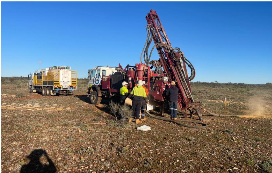
Figure 1: Aircore Drilling Rig at Everlong Prospect of the Austin Gold Project
