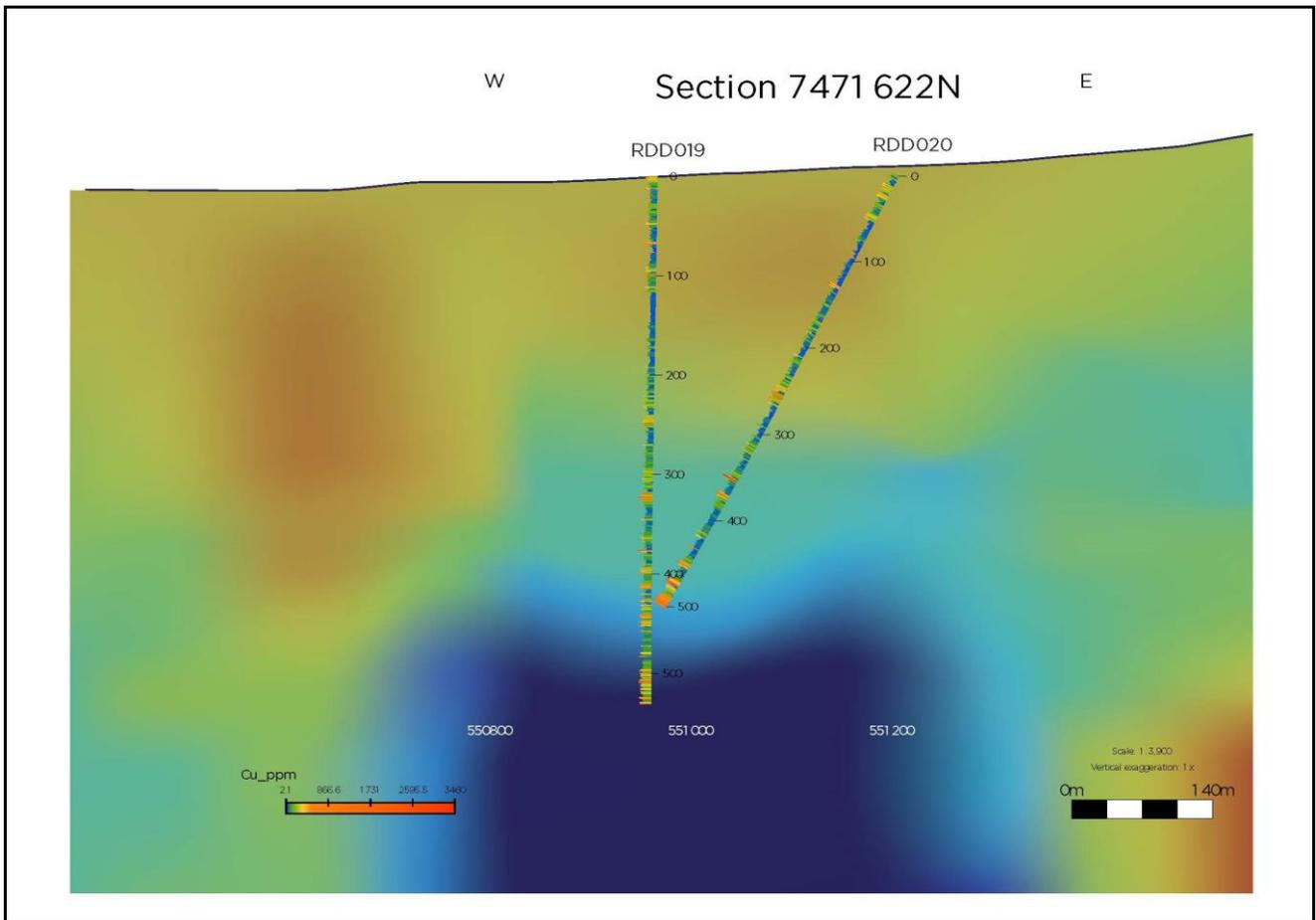
Figure 6. Idealised section projecting both holes onto the modelled magnetic low anomaly at the Clermont Porphyry Prospect
