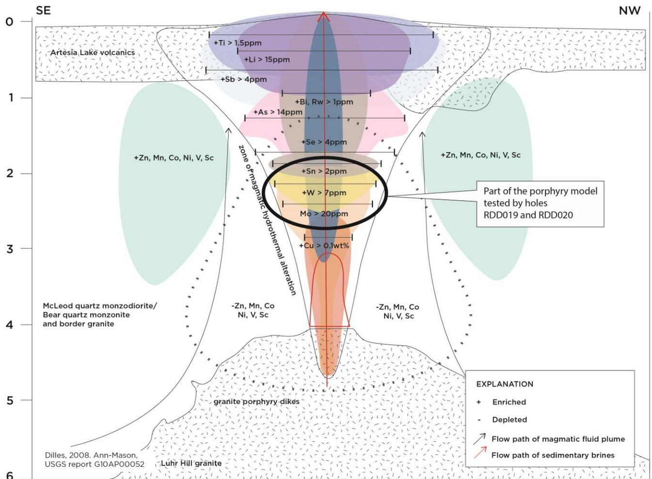
Figure 5. Drilling at the Clermont Porphyry Prospect and relationship to modelled porphyry geochemistry (from the Ann-Mason copper porphyry - Nevada)
