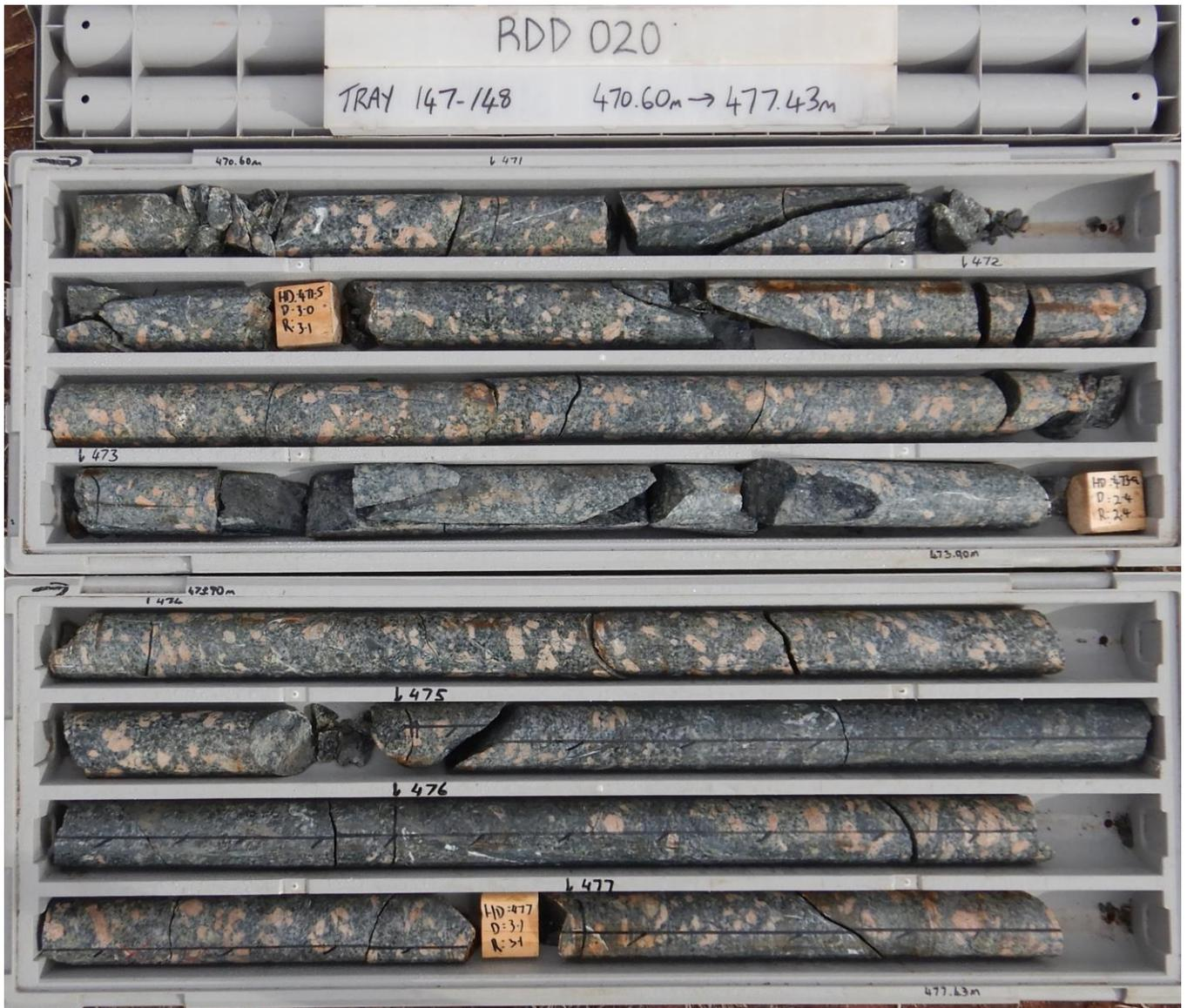
Figure 4. RDD020, 2m @ 1.69g/t Au, 2.22g/t Ag and 0.17% Cu from 475m
